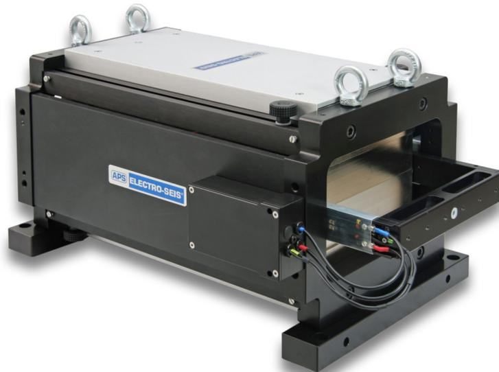
The **APS 420 ELECTRO-SEIS®** shaker is a long stroke, electrodynamic force generator specifically designed to be used alone or in arrays for studying dynamic response characteristics of various structures. It finds use in modal excitation of complex structures, particularly when low frequencies are required. Furthermore it can be used for low frequency vibration testing of components and assemblies.
